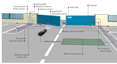
If a careful analysis of the automated gate's risks were to require it, the use of sensitive safety infrared or mechanical contact edges would become indispensable.
