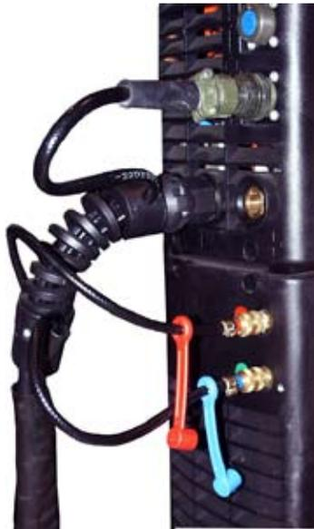
Installing water-cooled torch
